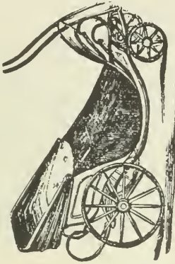
No. 17 is a four-wheeled Victoria Pleasure Chair, mounted in a very light iron framed carriage, upon c and patent India-rubber springs, is either drawn by hand or animal, and is the most elegant and easiest chair made.
